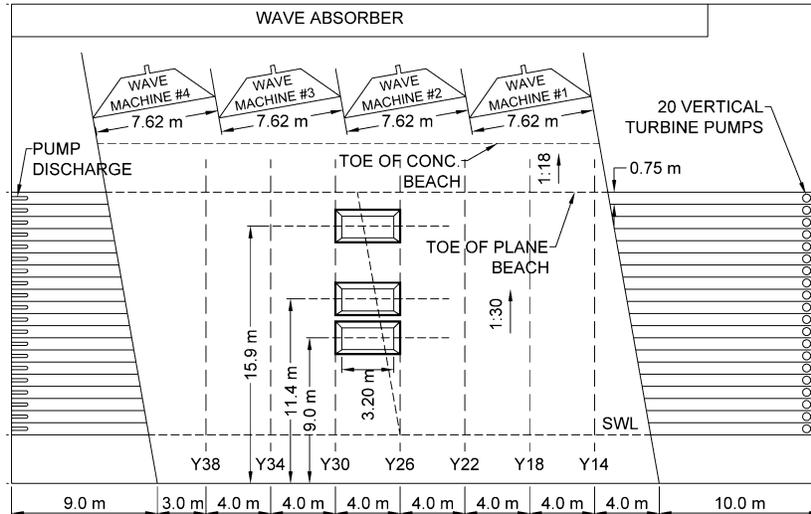
**Figure 1. Large-scale Sediment Transport Facility layout with berm dimensions.**
