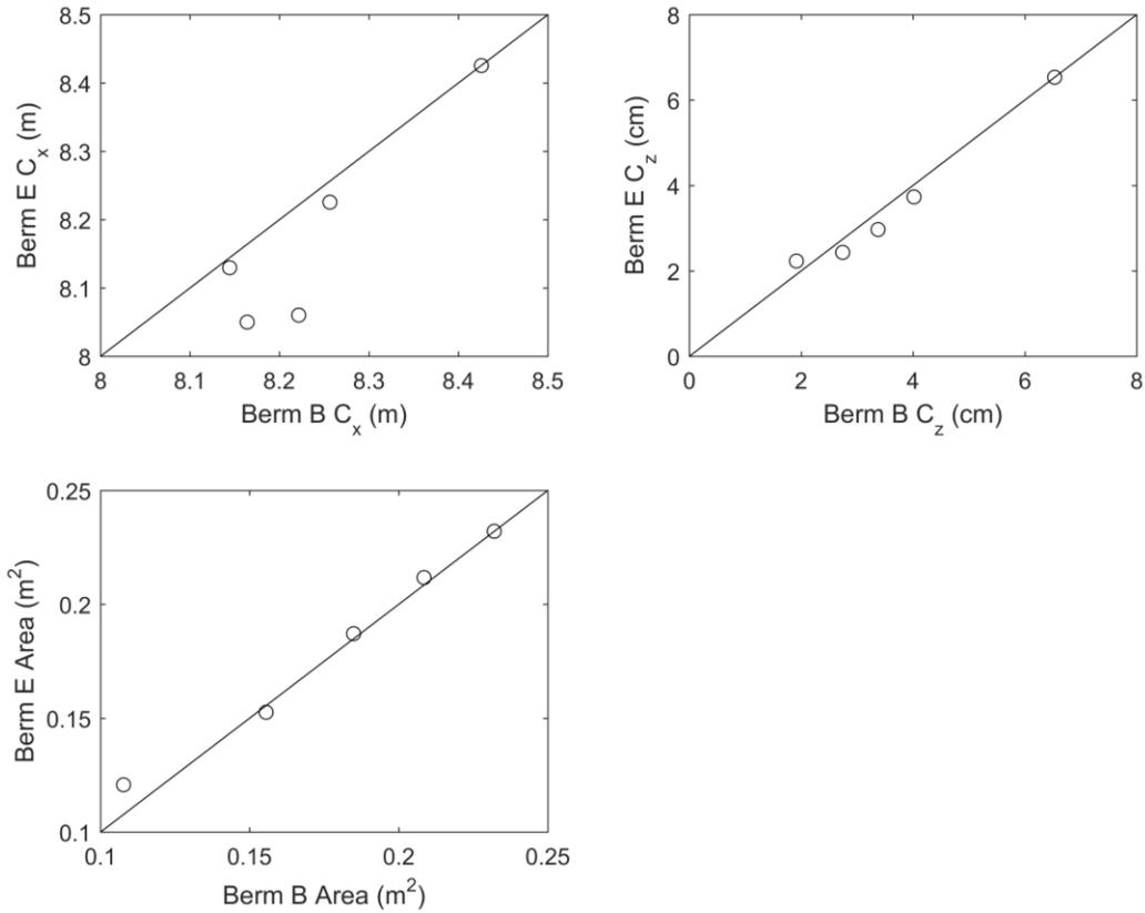
Figure 4. Comparisons for cross-shore centroid, vertical centroid and berm area of identically built nearshore berms with an incident wave height,  $H_{m0} = 21.4$  cm and  $T_p = 3.5$  s.
