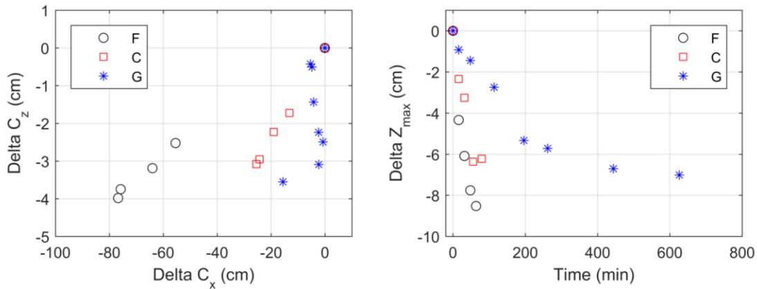
Figure 7. Change in centroids ( $C_z$  and  $C_x$ ) and maximum berm height ( $Z_{max}$ ) for Berm C, F, and G.
