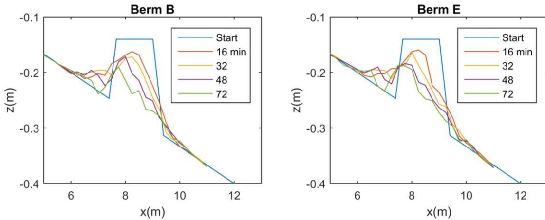
**Figure 3. Evolution of identically built nearshore berms for presented forcing intervals with an incident wave height,  $H_{m0} = 21.4$  cm and  $T_p = 3.5$  s.**
