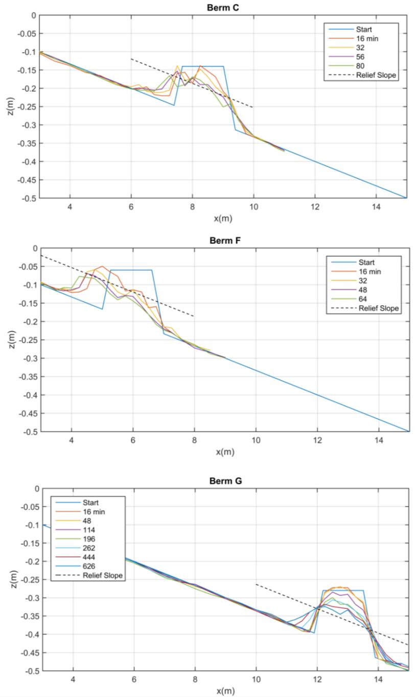
Figure 6. Measured centerline cross-shore profiles for Berm C, F, and G.
