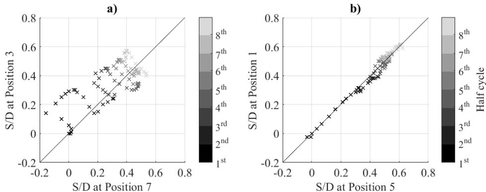
**Figure 7: Comparison of scour depth for a) measurement positions in streamwise direction and b) lateral direction for test case Tide\_02. The colorbar shows the development of scour depth over the individual tidal half cycles.**
