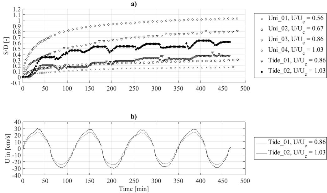
Figure 9: Development of maximum scour depth over time for unidirectional and tidal test cases. b) ADV velocity measurements for both tidal test cases.
