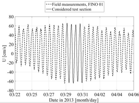
Figure 2: Velocities measured at half water level.
