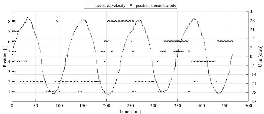
**Figure 8: Variation of position of maximum scour depth at the pile over time for the Tide\_02 test case in comparison to ADV velocity measurements for Tide\_02.**
