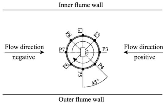
**Figure 5: Positions for scour measurement around the pile in top view.**
