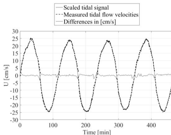
Figure 4: Comparison of measured velocities for tidal test Tide\_01 with a peak velocity of  $U_{peak} = 25.3$  cm/s and the corresponding original scaled field data.
