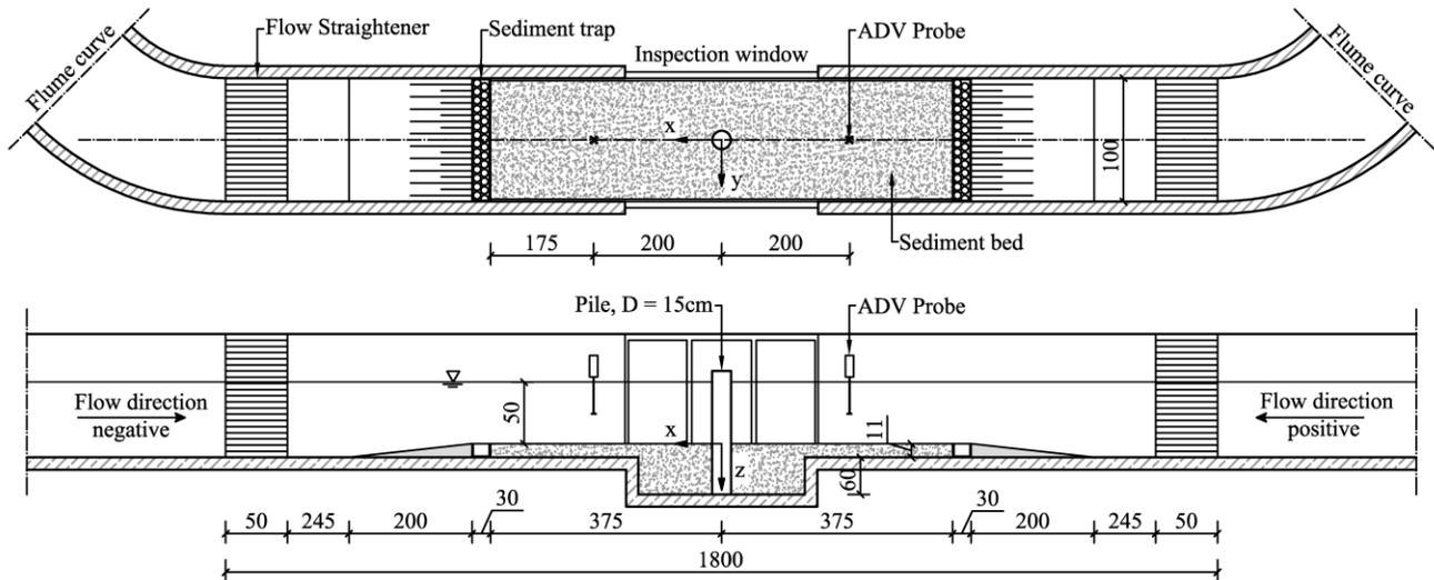
Figure 1: Schematics of experimental setup in top and side view with numbers in centimeter (not to scale).
