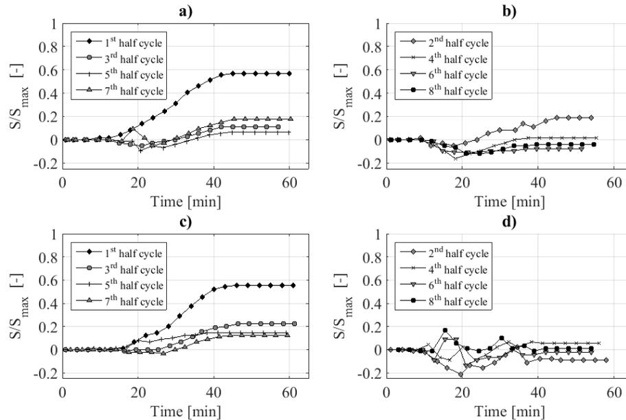
Figure 10: Comparison of scour development for each tidal half cycle with  $S/S_{max}$  as the ratio of the maximum scour depth in a half cycle to the final scour depth at the end of the test case. a) Scour development in Tide\_02 for positive flow direction and b) for negative flow direction. c) Scour development in Tide\_01 for positive flow direction and d) for negative flow direction.
