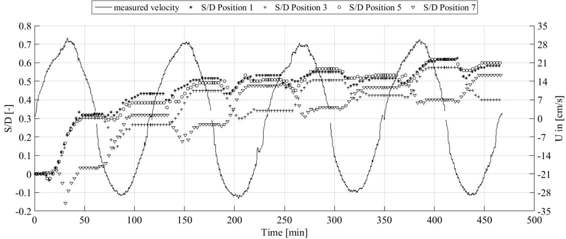
**Figure 6: Scour development at the streamwise (position 3 and 7) and lateral (position 1 and 5) positions around the pile for Tide\_02 with a maximum  $U/U_c = 1.03$  in comparison to ADV velocity measurements at half water depth for Tide\_02.**
