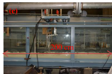
Fig. 1 Sketch of the wave flume experimental setup (dimensions in m)
