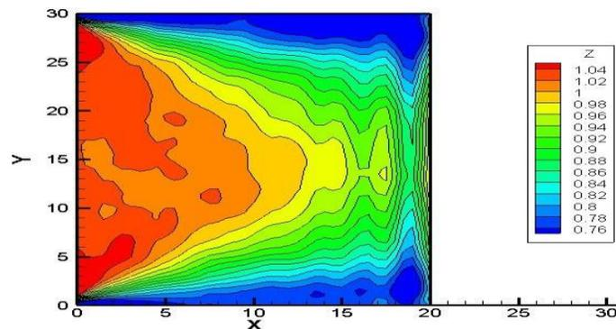
**Figure 5 Normalized significant wave heights for irregular multidirectional waves**
