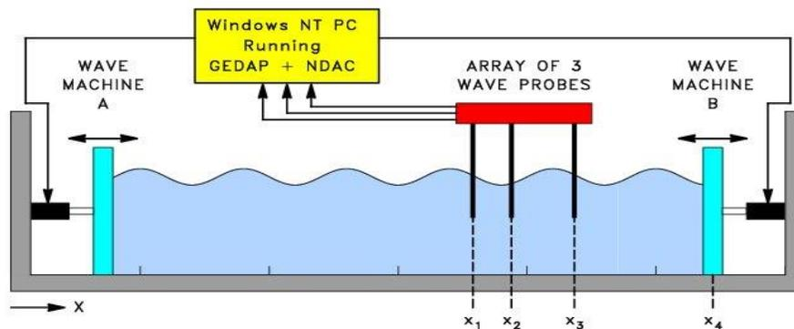
**Figure 2. Layout of the special wave flume for validation of active wave absorption techniques**
