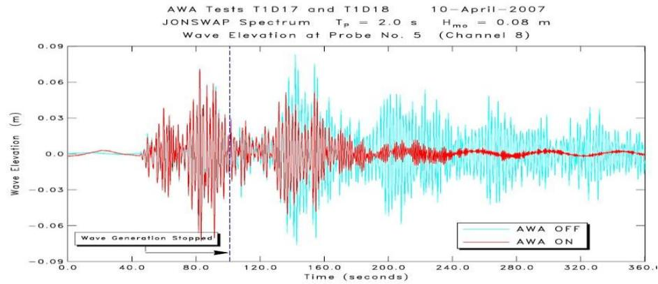
**Figure 3. Validation of the active wave absorption technique**
