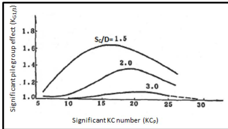
Figure 7. Relationship Pile group effect  $K_G$  for middle pile in side by side arrangement for pure-wave condition (Li et al., 1993)
