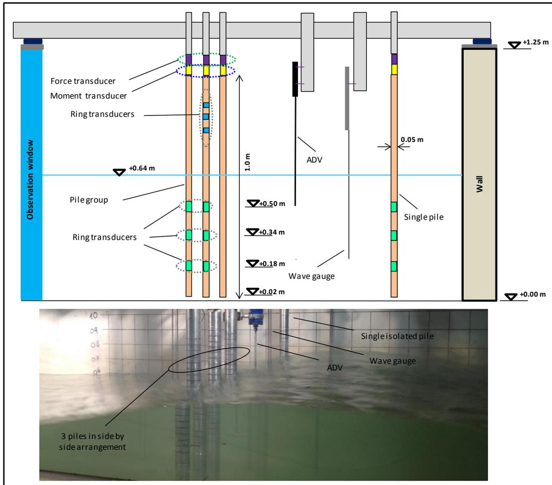
**Figure 4. Cross-section and a snapshot of model set-up of LWI tests, exemplarily for a pile group with side by side arrangement**
