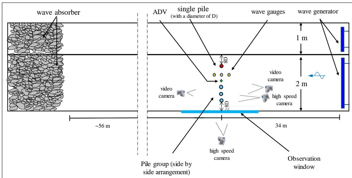
Figure 3. Plan view of model set-up of LWI tests, exemplarily for a pile group with side by side arrangement
