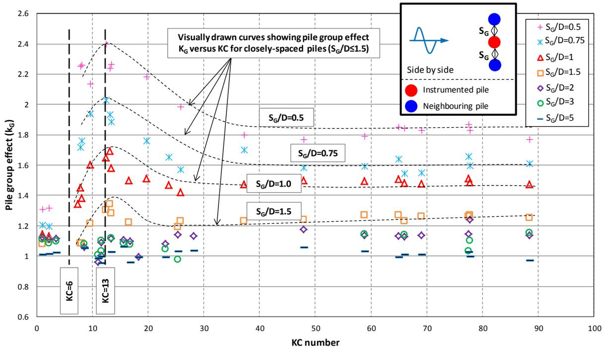
Figure 6. Relationship between pile group effect  $K_G$  and  $KC$  number for side by side arrangement exposed to regular non-breaking waves
