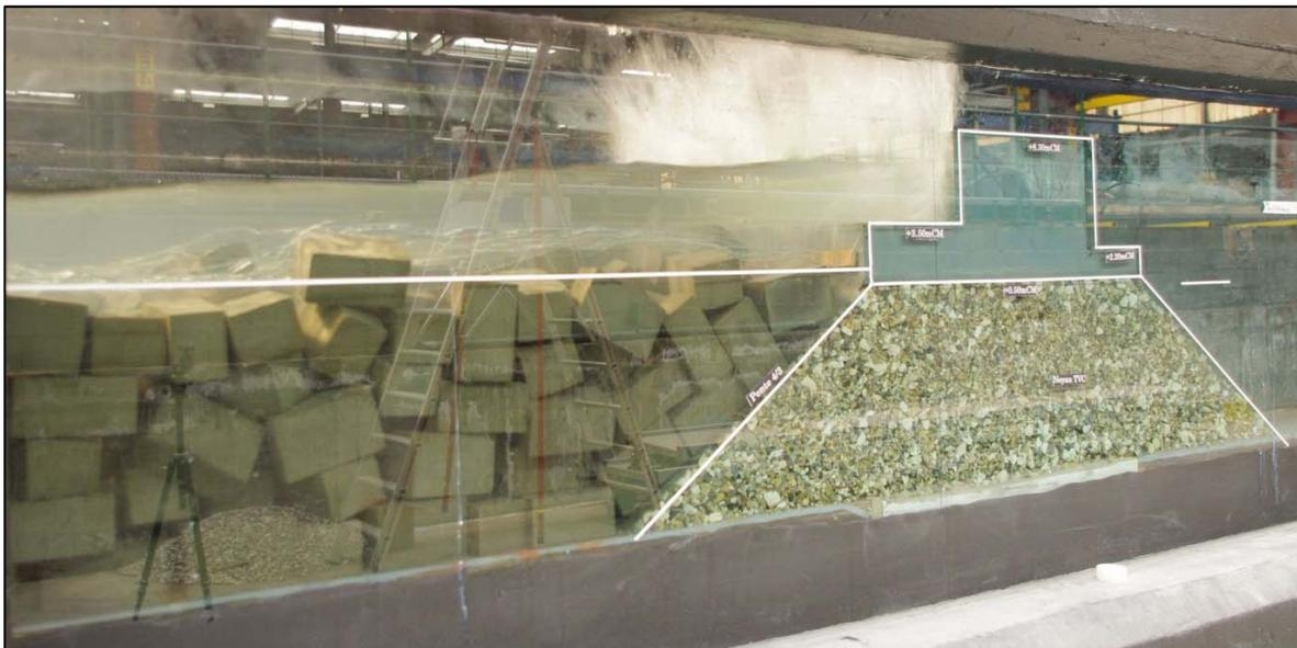
**Figure 6. Side view of the model of the Artha breakwater during regular wave testing (measurement of pressures and forces on the wall), water level: +4.30mCD, T=16s, H=6m.**
