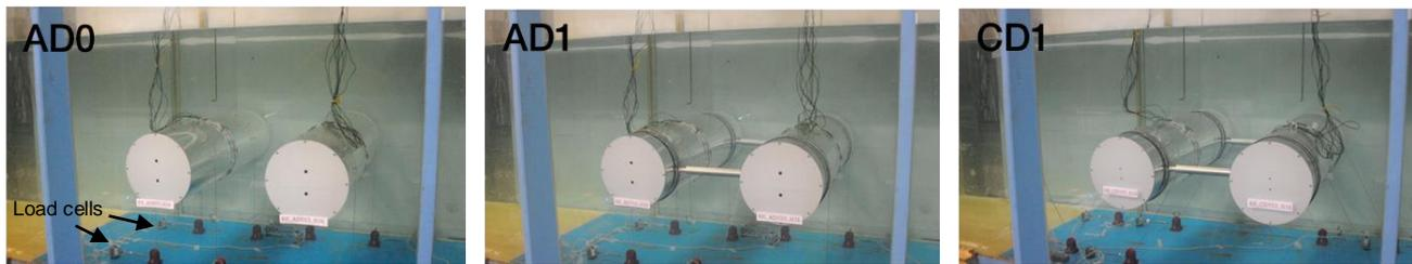
Figure 2. Three different configurations of the twin SFT model installed in the wave flume
