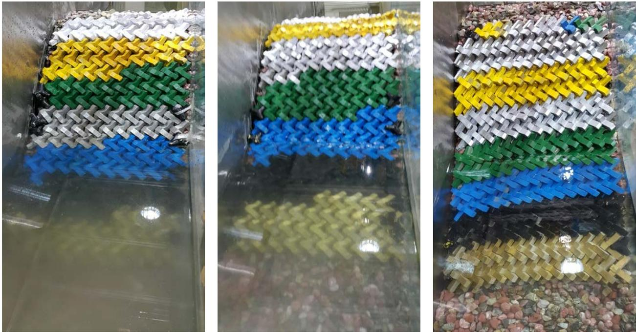
**Figure 8. Chi blocks for uniform placement after experiments (Chi block 1(Left) to Chi block 3(Right))**
