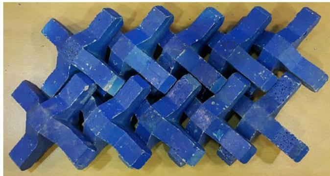
**Figure 3. The method of placement for Chi blocks (uniformly x-shape placement in single layer)**
