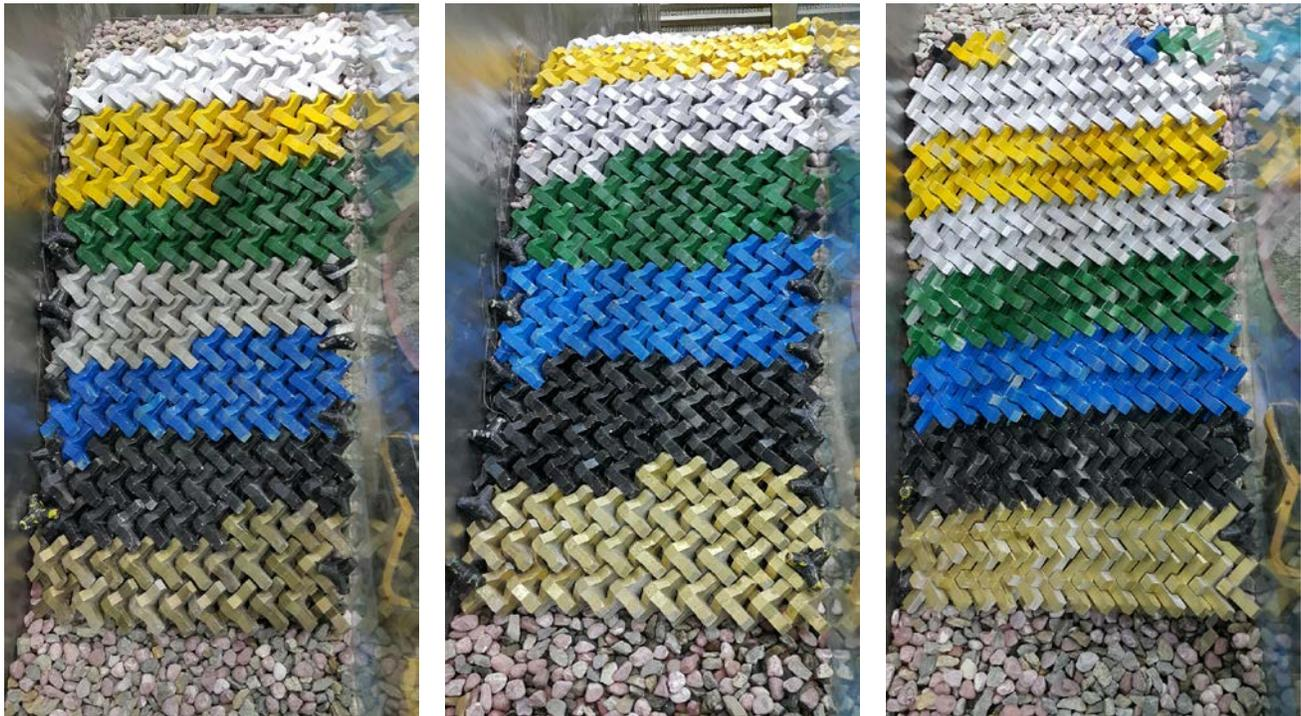
Figure 6. Chi blocks in a uniformly x-shape on the filter layer (Chi block 1(Left) to Chi block 3(Right))
