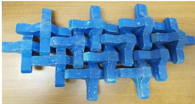
**Figure 2. The method of placement for Chi blocks (uniformly + shape placement in single layer)**
