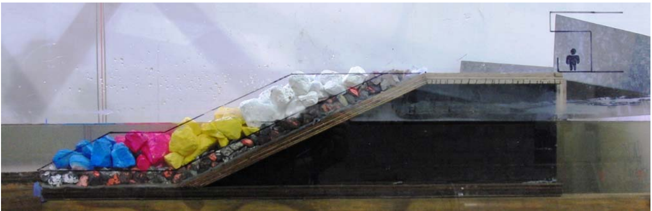
Figure 3. Example photograph of model structure prior to testing in the 2D wave flume (7 t rock, 1V:2.2H slope, no wave return)
