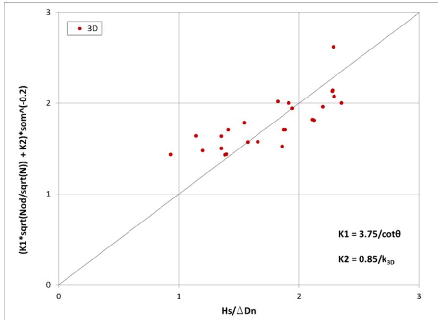
Figure 15. Comparison of  $N_s$  and the right-hand-side of Equation 12 for the basin results (3D)
