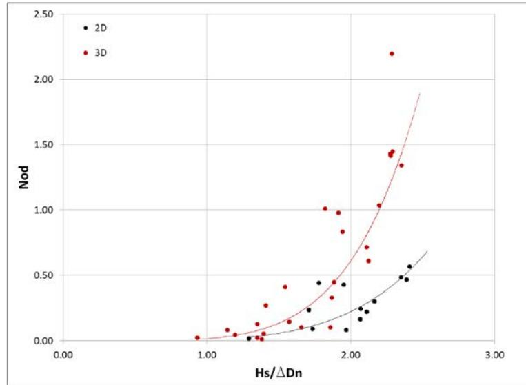
Figure 7. Comparison between  $N_s$  and cumulative relative damage for all test results
