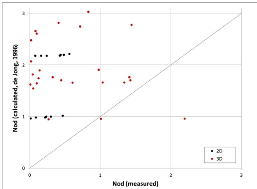
Figure 14. Measured cumulative relative damage versus cumulative relative damage from de Jong, 1996
