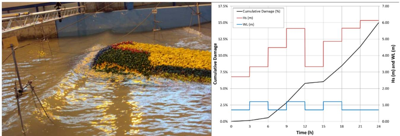
Figure 5. View of 3D model under wave action (IH Cantabria) Figure 6. Example of a design storm tested in 3D basin
