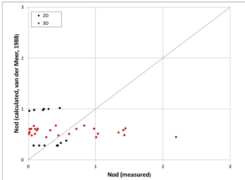
Figure 13. Measured cumulative relative damage versus cumulative relative damage from van der Meer, 1988
