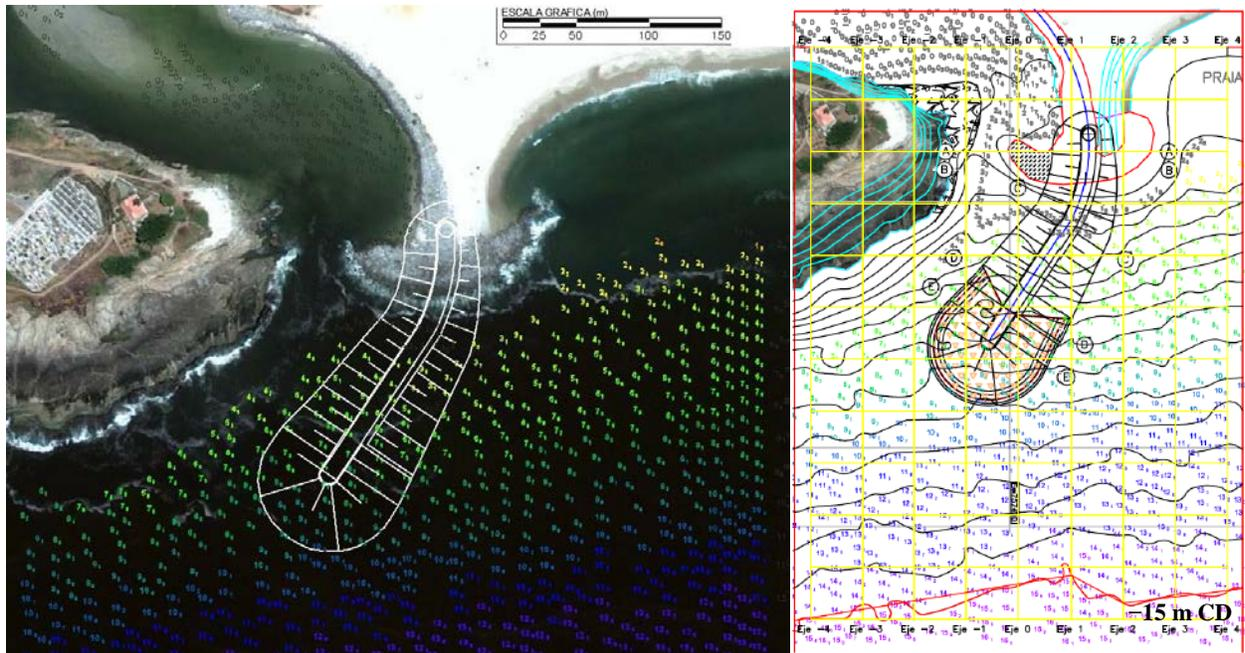
Figure 4. Site bathymetry: 2013 survey (left) and 3D wave basin grid (right), both in m referred to CD.
