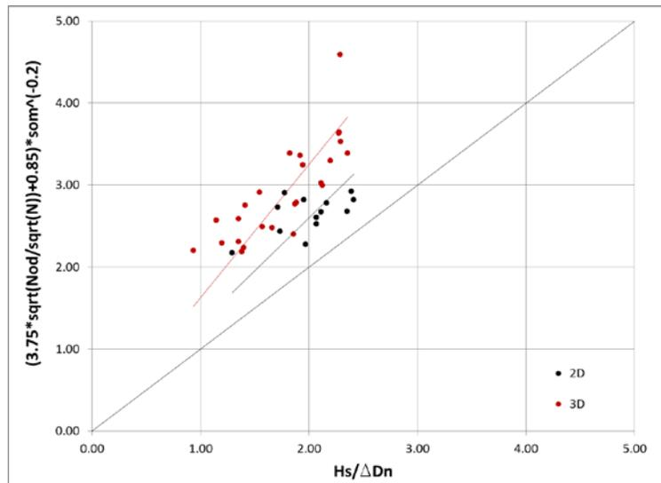
Figure 10. Comparison of  $N_s$  and the right-hand-side of Equation 3 (van der Meer, 1988)
