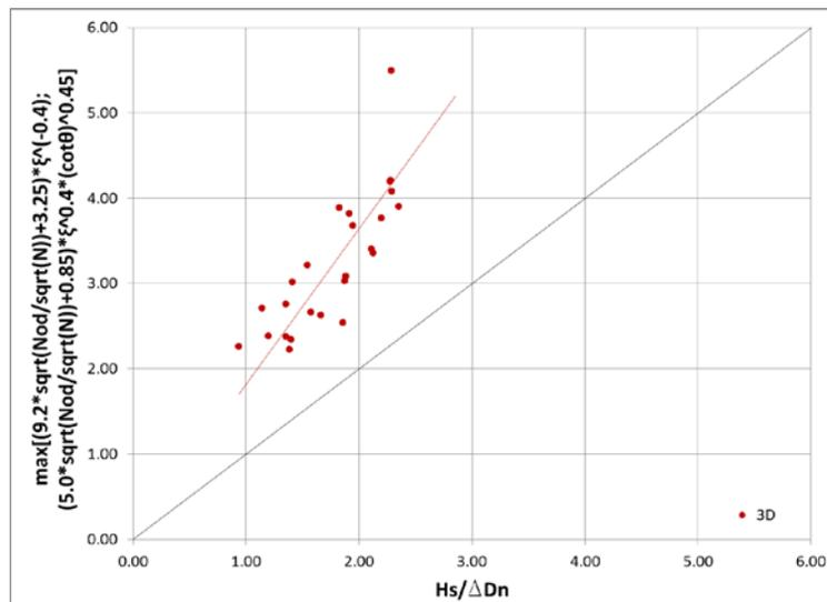
Figure 12. Comparison of  $N_s$  and the right-hand-side of Equation 9 (Suh and Kang, 2012) for 3D results
