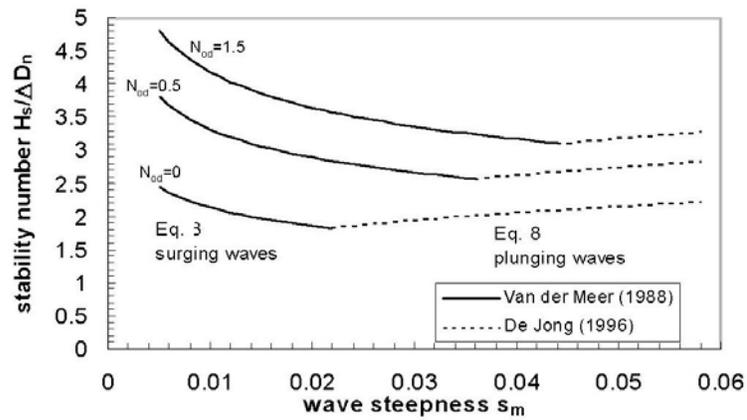
Figure 8. Wave steepness ( $s_{om}$ ) and Stability Number ( $N_s$ ) for tetrapods (from van der Meer, 1999)
