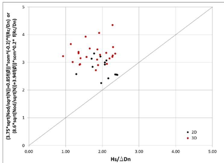
Figure 11. Comparison of  $N_s$  and the right-hand-side of Equations 4 and 8 (de Jong, 1996)
