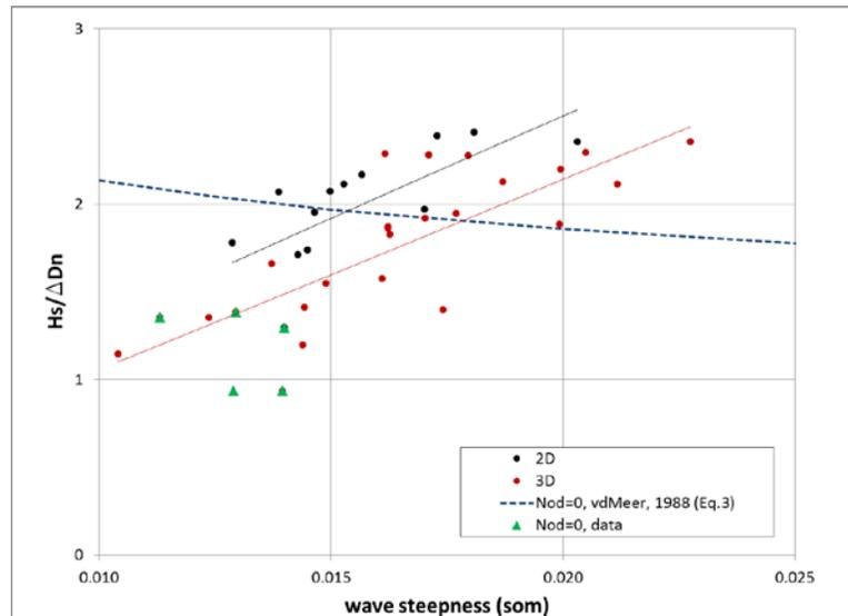
Figure 9. Comparison between wave steepness  $s_{om}$  and Stability Number  $N_s$  (2D and 3D data)
