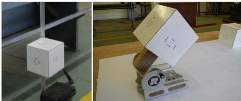
Figure 5. Vertical guide used for heave accuracy tests (left). Adjustable bracket for pitch and roll accuracy tests (right)
