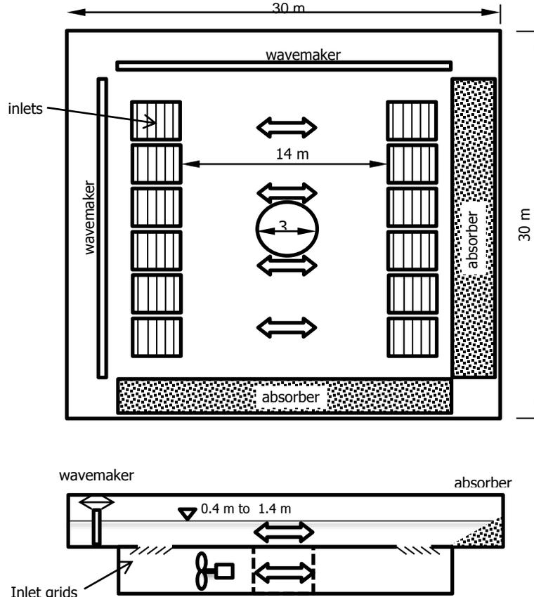
Figure 3. COB schematic including the wavemaker and the current system (top: plan view, bottom: cross section).
