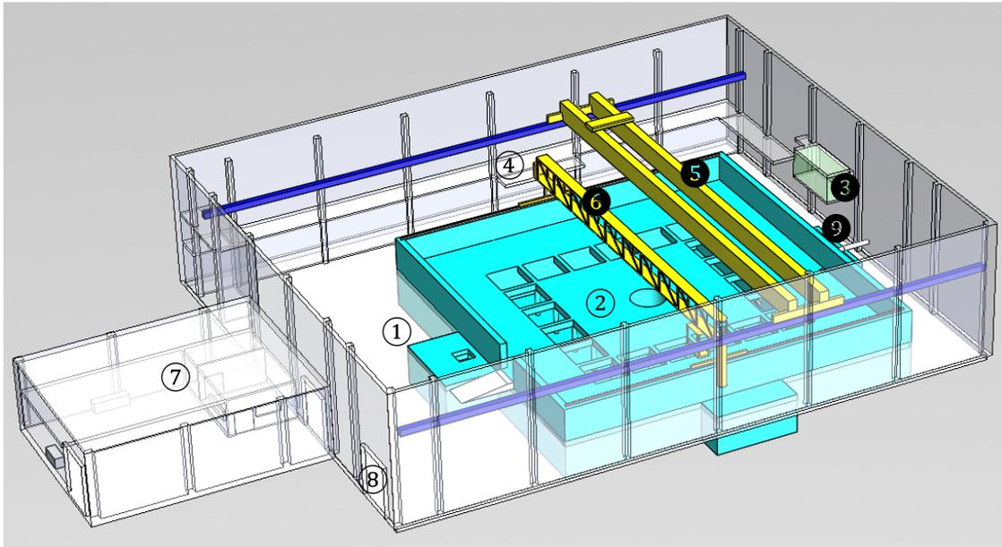
**Figure 2. Overview of the COB facility: 1) COB lab, 2) COB, 3) Main operation location, 4) Secondary operation location, 5) Bridge crane, 6) Carriage (access bridge), 7) Workshop, 8) External access, and 9) Water transfer system.**
