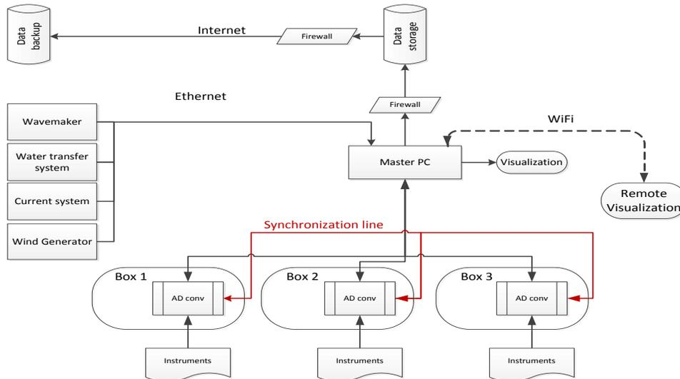
Figure 7. Schematic of the planned data acquisition system in the COB.
