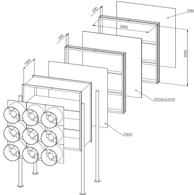
Figure 5. Wind Generator exploded view.
