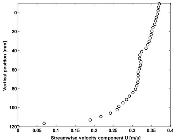
Figure 4. Velocity profile in model current system.
