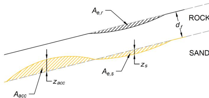
Figure 3. Erosion and accretion pattern (parameter definition).
