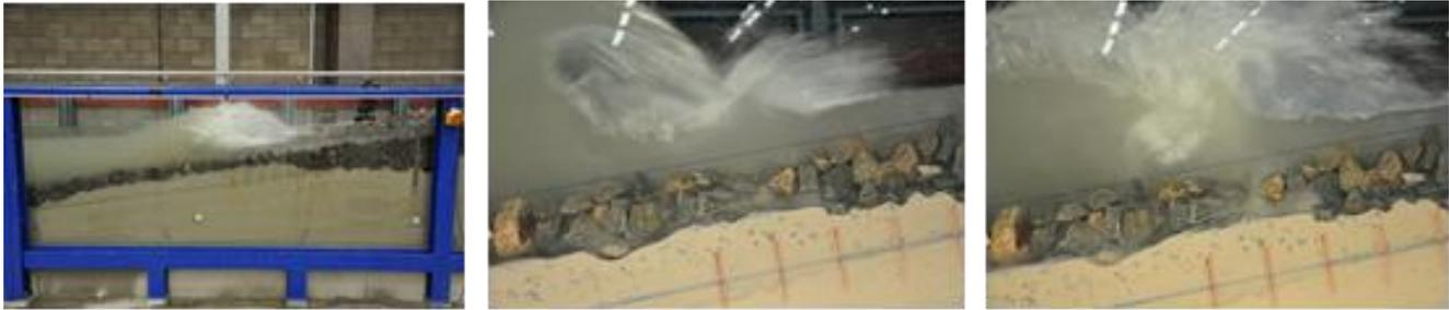
**Figure 1. Physical model tests with open transport filters with rock on top of sand (from Van Gent and Wolters, 2015).**
