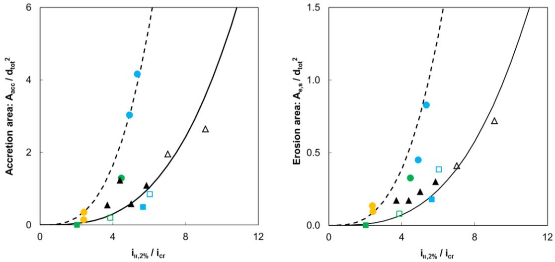
Figure 5. Sand accretion and erosion: Area of accretion (left) and erosion (right) versus the hydraulic gradients at interface.
