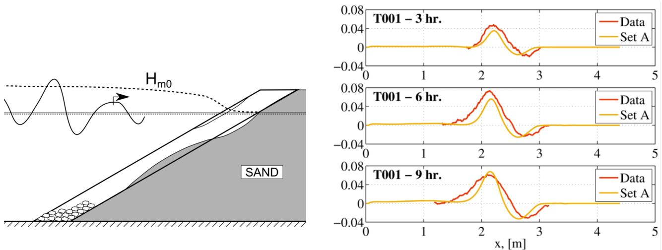
**Figure 9: Left: Schematised configuration in numerical model (1:4 slope). Right: Comparison of measured versus calculated deformed internal rock-sand interface (deformation in [m] on vertical axis) (courtesy Jacobsen et al., 2016).**
