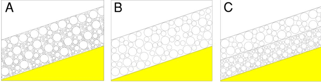
Figure 2. Tested configurations of the open filter (rock on top of sand).
