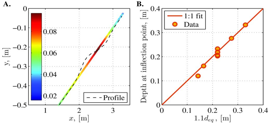
**Figure 8:** Left: Location of calculated hydraulic gradients and the measured inflection point. Colours indicate the magnitude of hydraulic gradients and the dashed line the measured profile. Right: The water depth at the maximum value of hydraulic gradients as a function of the layer thickness (from Van Gent *et al.*, 2015).
