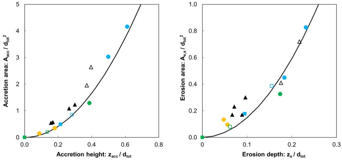
Figure 4. Sand accretion and erosion: Observed relation between area and height of accretion (left) and erosion (right).
