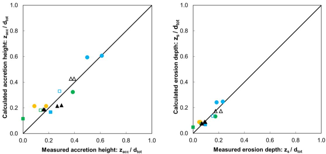
Figure 6. Sand accretion and erosion: Comparison of measured and calculated accretion (left) and erosion (right).
