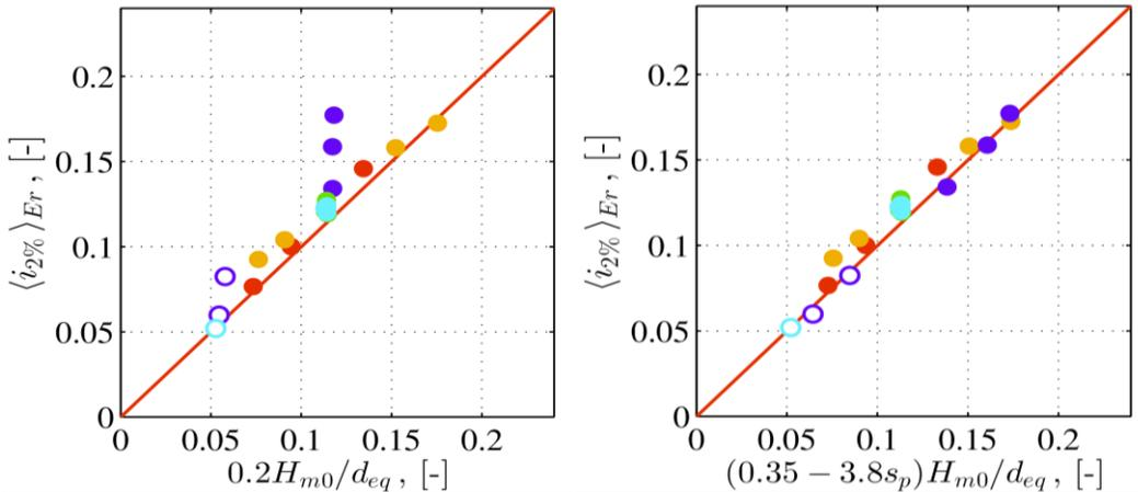
**Figure 7: Left: Calculated hydraulic gradients in the area of erosion versus the expression derived from experiments. Right: Calculated hydraulic gradients versus an extended expression including the wave steepness (from Van Gent *et al.*, 2015).**
