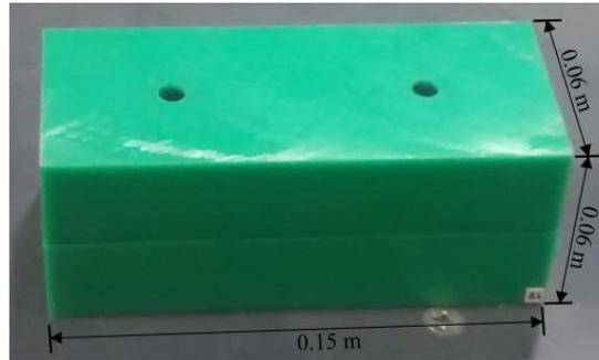
**Figure 2. Idealized Shipping Container Model used as Debris (Scaled-down 20-foot shipping container).**
