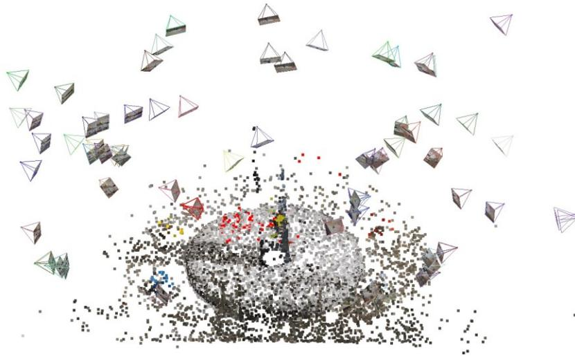
Figure 5. Positions of images used in the SfM method
