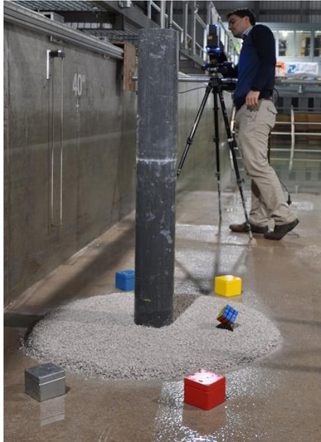
**Figure 3. Operation of the TLS**
