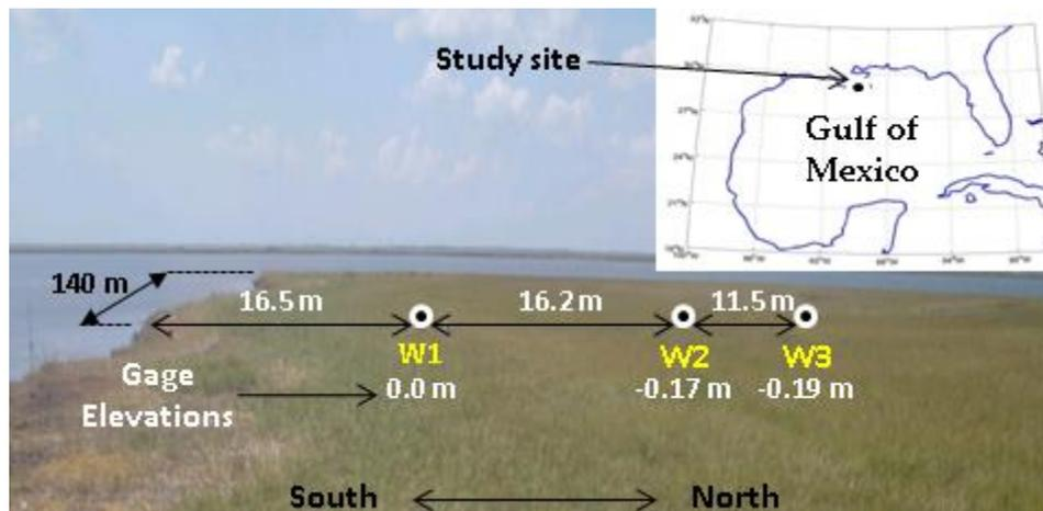
Figure 3. Study area location (Terrebonne Bay, Louisiana) and the schematic of experimental set up showing wave gages (W1-W3). Gage elevations relative to gage W1. Not to scale.
