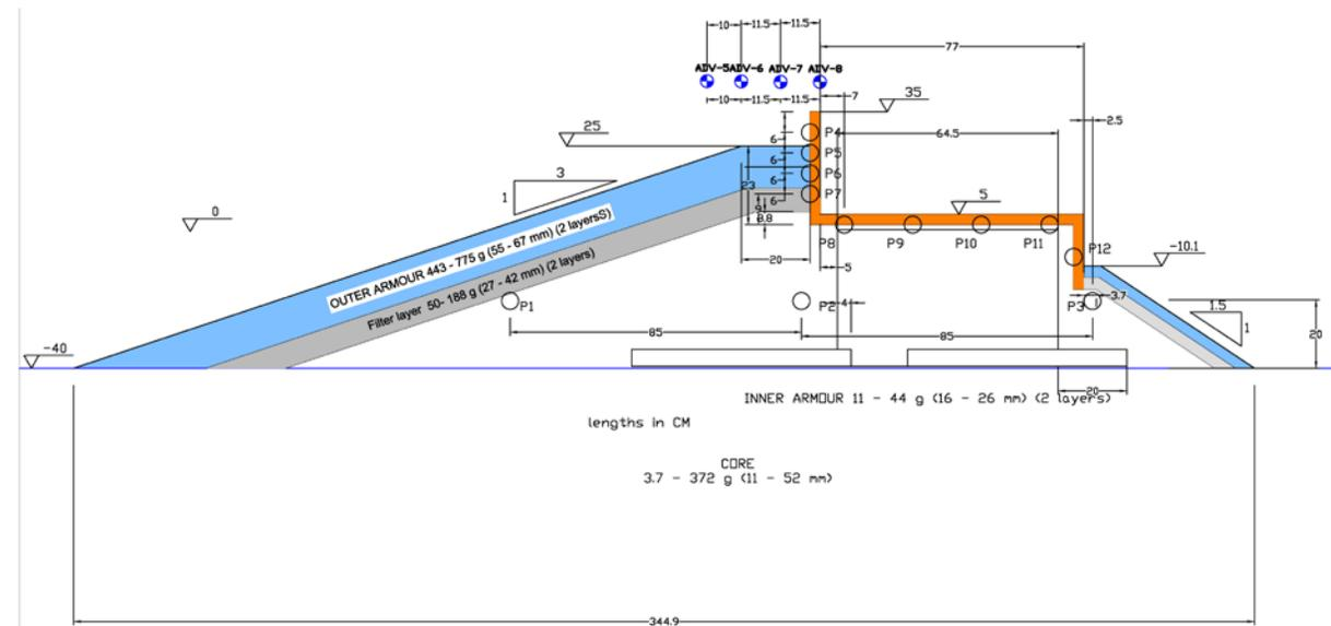
Figure 4. Rubble-mound breakwater with crown-wall (type I) transversal section
