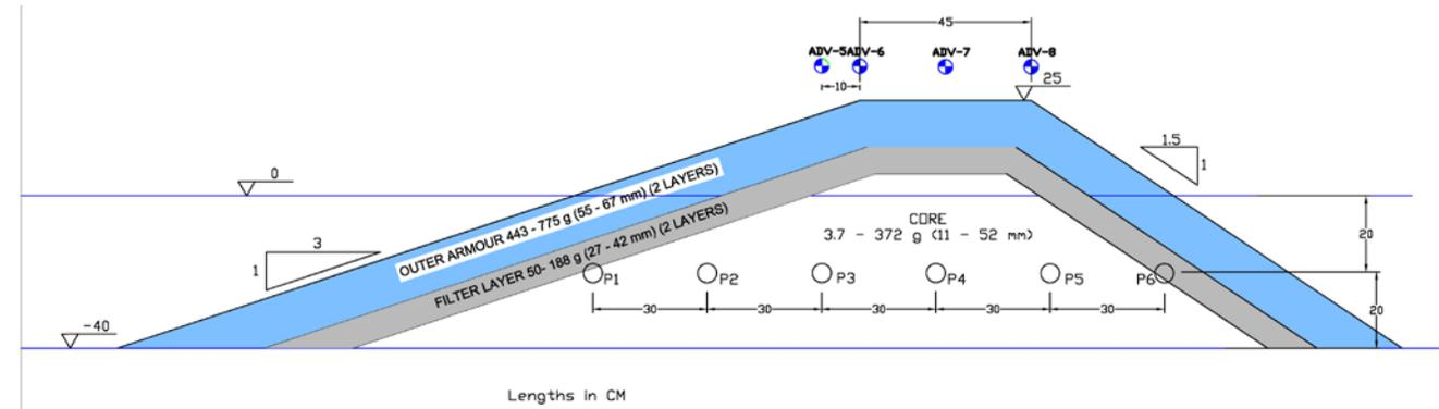
**Figure 5 Rubble-mound breakwater without crown-wall (type II) transversal section**
