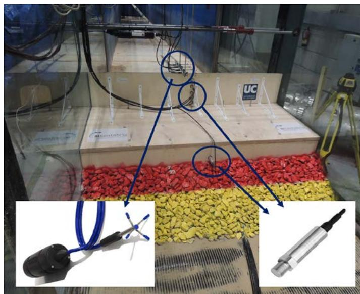
Figure 7. Some of the pressure gauges and a horizontal array of ADVs from the leeside of the breakwater type I during its construction
