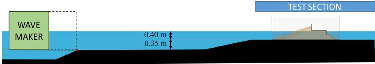
Figure 3. Schema of the wave flume, including the test section
