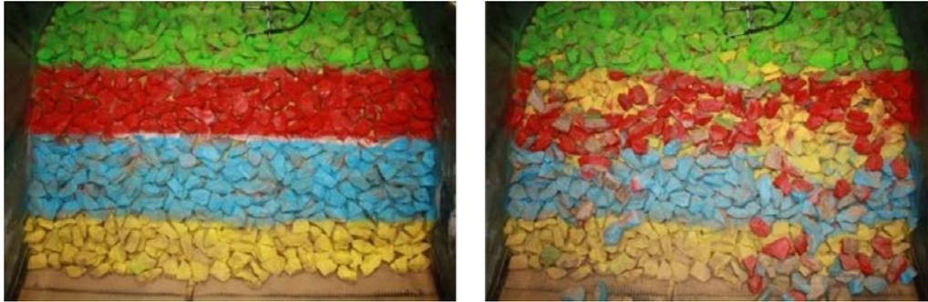
**Figure 8. Layers painted in different color to help the visualization and identification of the armor damage and the counting of moved stones, before and after a solitary wave test, breakwater type II.**
