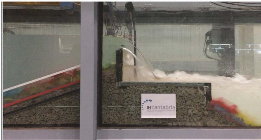
**Figure 9. Overtopping over RMB with crown wall**
