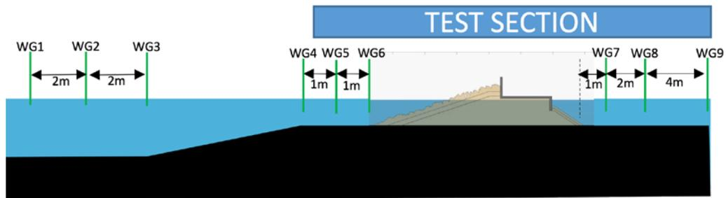
Figure 6. Scheme of the position of the wave gauges (WG) in the flume
