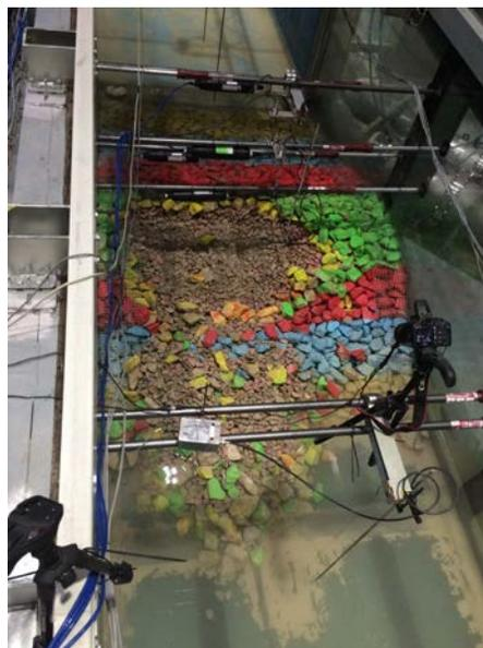
**Figure 11. Top view of the type II model damage after overflow tests**
