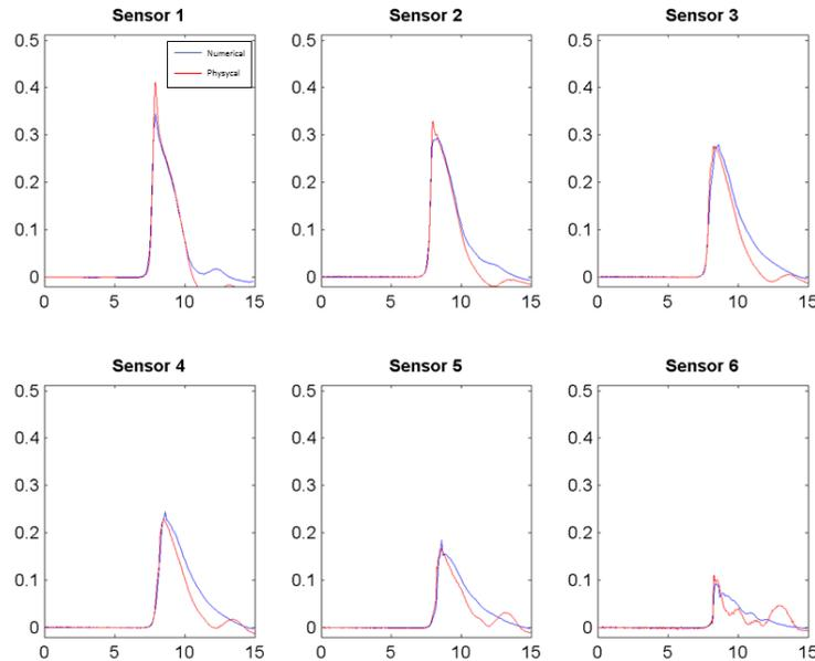
**Figure 12. Comparison between physical and numerical experiments. Pressure in the core of RMB type 2 for a 0.4m Solitary Wave**
