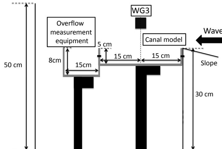
Figure 3. Canal model and overflow measurement equipment.
