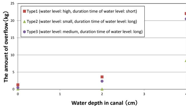
Figure 7. The difference between the amount of overflow and water depth in canal.
