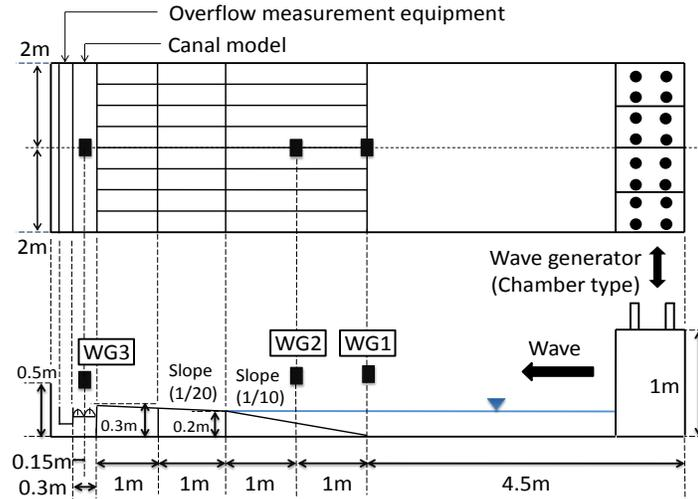
Figure 2. Experimental layout in a tsunami basin.
