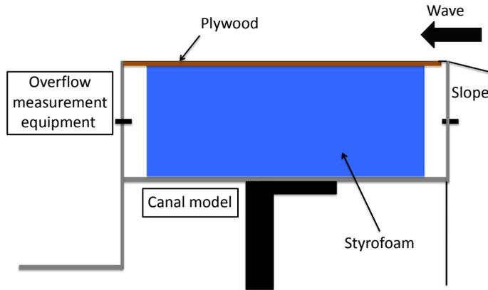
Figure 4. The experimental condition without canal.
