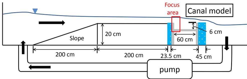
Figure 8. Experimental layout in a wave flume.
