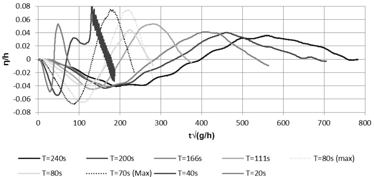
Figure 7 Calibrated N-waves using 2<sup>nd</sup> generation TS, measured at the toe of the bathymetry (WG\_05).
