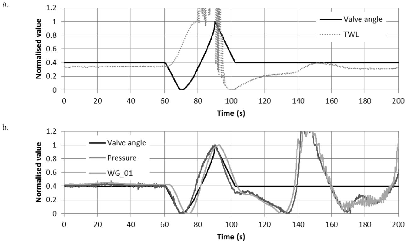
Figure 11 Normalised valve time series with the normalised TWL (a) and normalised valve time series with tank pressure transducer and WG\_01 free-surface elevation (b) for  $T=40$ s N-wave. All normalised using the primary peak and trough of the signal, ignoring additional reflections
