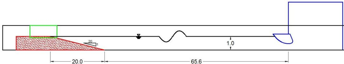
**Figure 4 Schematic of 2<sup>nd</sup> generation Tsunami Simulator setup showing the Tsunami Simulator with the flow shaper at the outlet, bathymetry and window position.**
