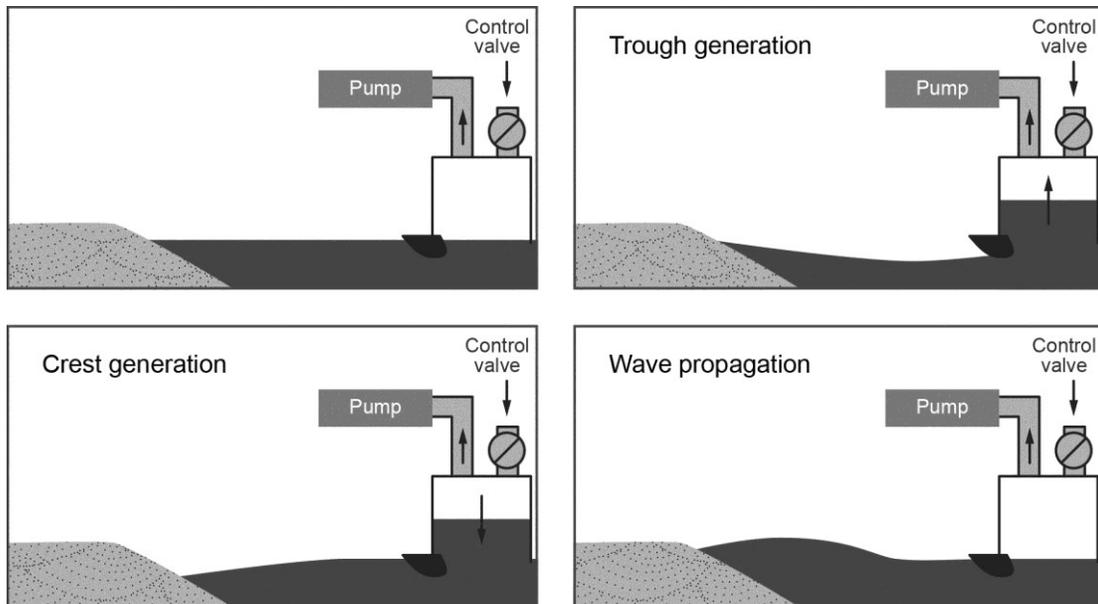
Figure 2 Schematic diagram of pneumatic Tsunami Simulator.
