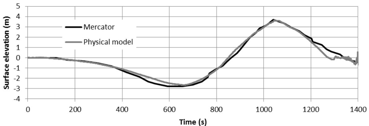
Figure 3 Reproduction of Mercator time series at 1:50 scale with 1<sup>st</sup> generation Tsunami Simulator.
