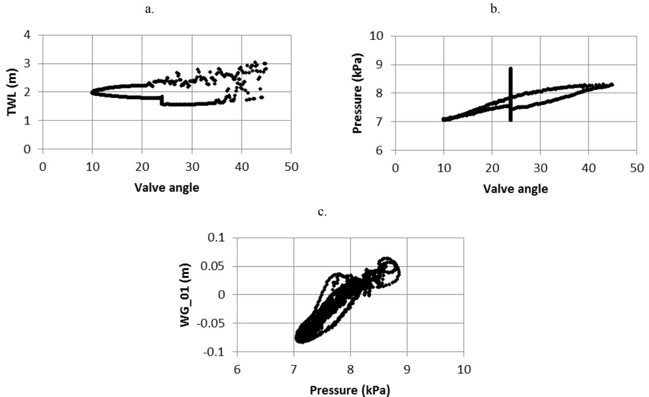
**Figure 12 Comparison of time co-incident values for a) valve angle and tank water level, b) valve angle and pressure at the base of the TS and c) pressure at the base of the TS and free-surface elevation at WG\_01.**
